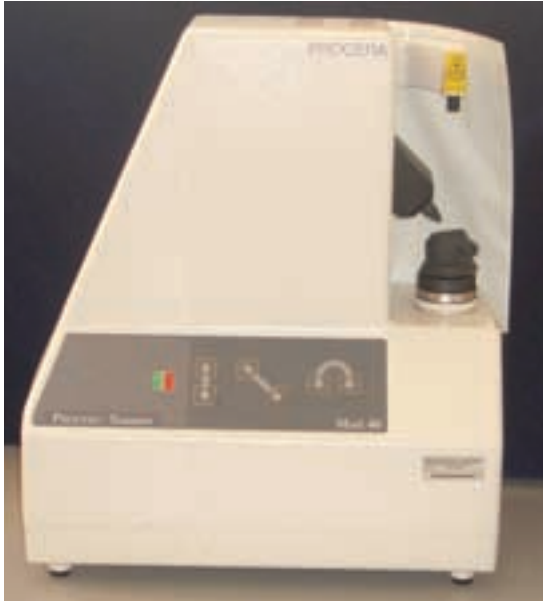
d The scanner used in the process of making a Procera crown.
